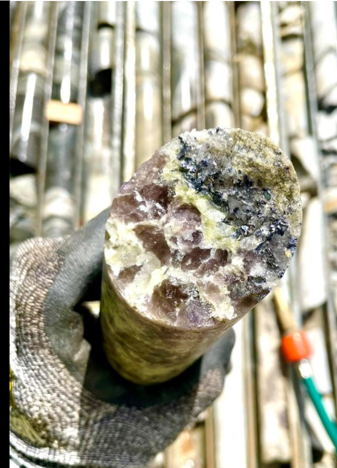
Coarse grained fluorite (purple) with wolframite (black) and molybdenite (silver) with quartz ± carbonate ± sericite
