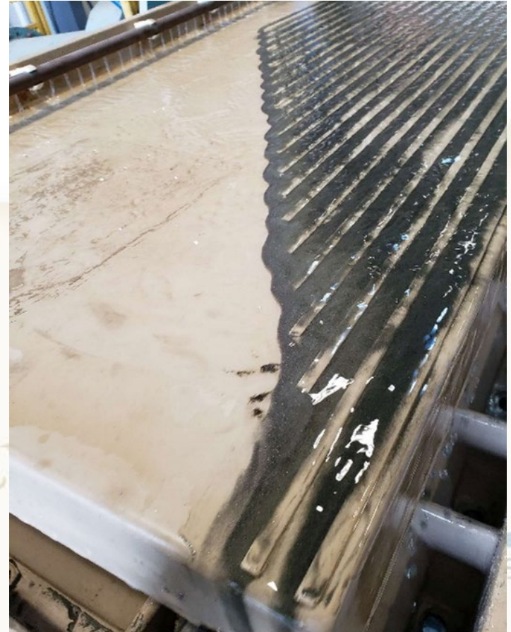
Tin Gravity Concentration on a Wilfley Shaking Table
